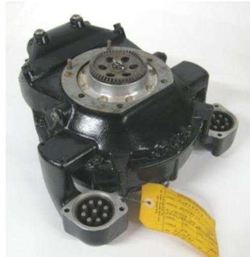
The picture on the left is of the Pratt and Whitney Double Wasp R2800 engine that's installed on the C46 and the picture on the right is that of the General Electric Magneto that powers the spark plugs.
